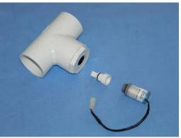
Note: If your mixing stick is built from something other than 1-1/2 inch PVC, you can purchase the correct size "T" at your local hardware store. Make sure that the part where the oxygen sensor goes has a ½" pipe thread. Remove the black sleeve from the provided 1-1/2" PVC "T" with your fingers. Do not use tools as you will mar the inside surface and the oxygen sensor/diverter will not fit or seal properly.
