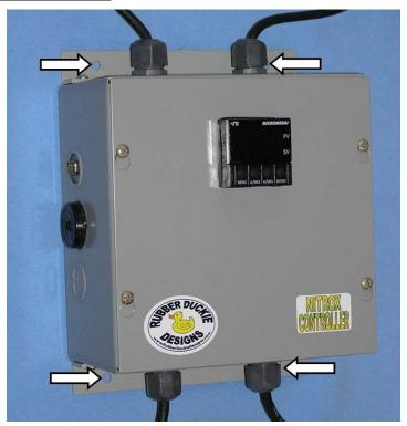
Note the four mounting holes on the Nitrox Controller mounting brackets. Position the controller at the desired mounting location and using a pen or pencil mark the four mounting holes on the wall. Carefully set the controller down out of the way.
